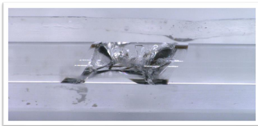
Figure 2. Excessive heating can cause fiber fuse type damage in FBGs.
