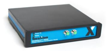
The ClearSpectrum™ TDCMB is a tunable, fully integrated emulator / compensator that provides accurate and dynamic control of chromatic dispersion for test and measurement applications. The instrument features TeraXion's fiber-Bragg grating (FBG) technology, which has a broad dispersion range and operational bandwidth. The TDCMB is available in benchtop and rackmount versions. The control software interface allows for easy integration and minimal setup time for experimental configurations.
